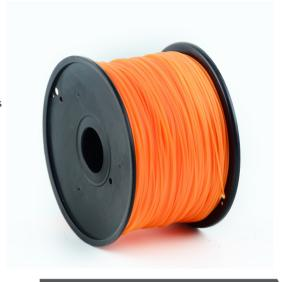
Material: PLA, 3 mm diameter Weight: 1 kg/spool (2.2 lbs) Length: approx. 120 m Density at 21.5?C: 1.25 g/cm3 Melt Flow Index at 10min, 2.16kg: 5
